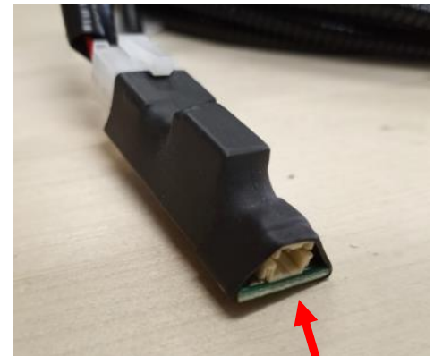
Plug OEM 2-Pin connector here
