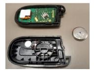
4. Remove the RAM overlay from the back of the key fob.
