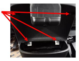
3. Mount the module in the location shown in the photo with screws and/or double-sided tape.
