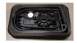
6. Flip the key fob and jig upside down and drill a hole through the back of the key fob using a 0.5" drill bit.
