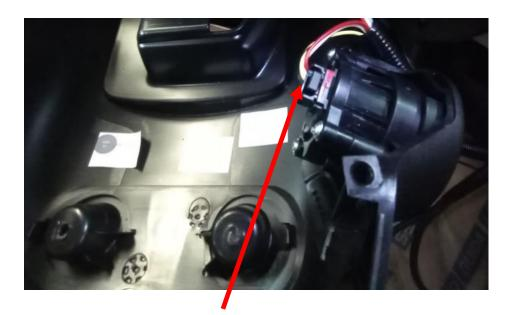
4. Remove the OEM connector from the rear of the Push-to-Start button and plug it into the mating connector on the InterMotive harness. Plug the male connector from the InterMotive harness into the mating connector at the rear of the Push-to-Start button.
