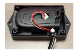
8. Place the top portion of the box on top and secure it with the four included screws. Plug the 3-pin connector into the mating connector on the main harness.
