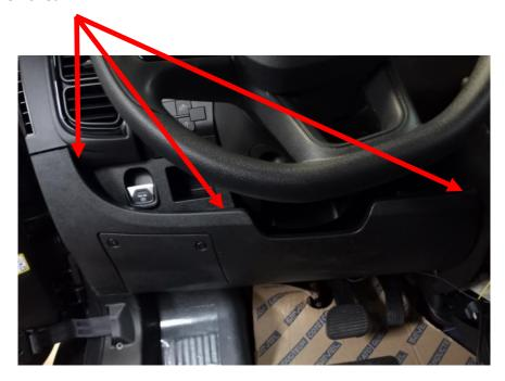
2. Remove the four screws attaching the lower shroud to the upper shroud.
