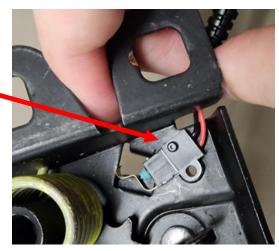
6. After the switch is properly positioned, fasten it down with the bolt, washer, and lock-nut.
