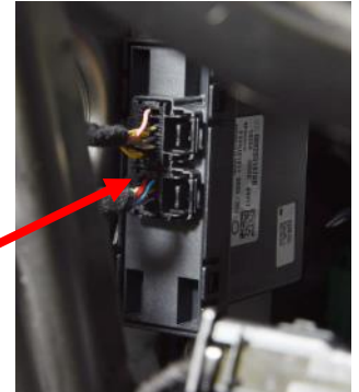
Charger gateway module with 8 & 12 pin connectors.
