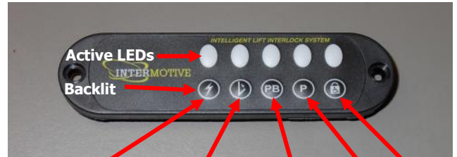
Vehicle Secure/Lift Enable, Lift Deployed, Park Brake, Park, Shift Lock
