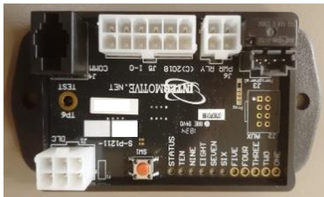
Data Link Harness plugs in here
