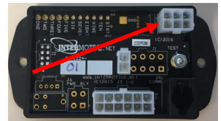
InterMotive Plug and Play Gateway Harness
