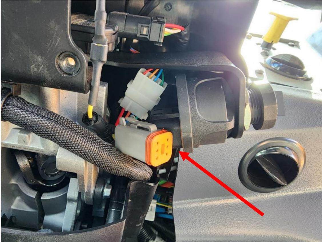
3. Plug the male Deutsch connector on the Intermotive 840-00411 harness into the ignition switch, and the female Deutsch connector into the male OEM connector.
