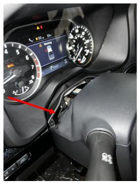
Remove the panel connected on the top side of the clamshell. The top and bottom shells can now be removed from each other.
