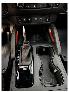
• Remove the metal pin in front of the knob and pull the knob up to separate.
