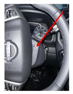
The 3rd screw is located underneath the clamshell.
