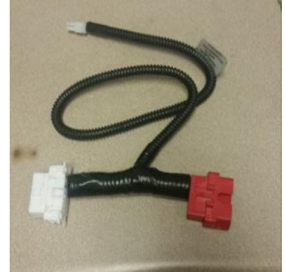
BOM Data Link harness "T's" into OBDII connector.
