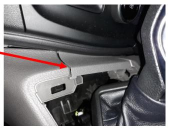
Remove the center under dash panel by firmly grasping it and pulling it towards the rear of the vehicle.
