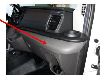
Open the glove box and remove the screw as shown in the photo
