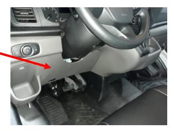
· Remove the two screws as seen in the photo
