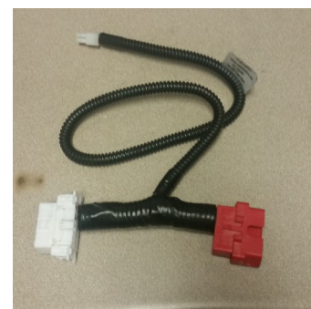
AFIS Data Link harness "T's" into OBDII connector.
