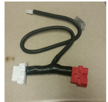
SBM Data Link harness "T's" into OBDII connector.
