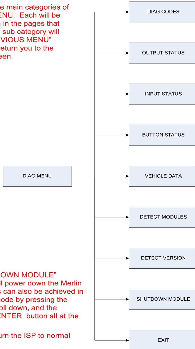
The "SHUTDOWN MODULE" command will power down the Merlin system. This can also be achieved in the normal mode by pressing the scroll up, scroll down, and the InterMotive/ENTER button all at the same time.
