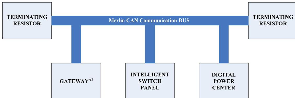
• Figure 1: Typical connection of the Merlin Multiplex System<sup>®</sup>
