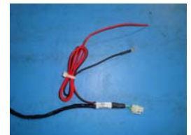
Merlin single piece harness with MIM connector & flying power leads on one end.
