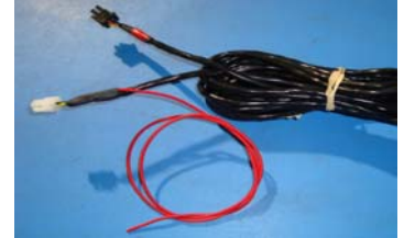
Merlin segmented harness with MIM connector & flying power lead on one end.
