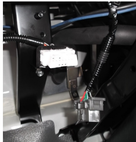
OEM OBDII bracket with White ITC950 connector installed, with Grey OEM connector in lower right
