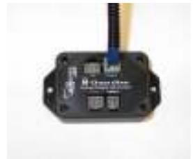
**LIFT HARNESS** – This harness can be identified by the green tape near the 6-pin connector. Attach the appropriate wheelchair lift adapter to the lift harness, then attach adapter to the wheelchair lift. Run the lift harness from the wheelchair lift to the Guardian Module. Finally, snap the green taped end of the Lift Harness into the Guardian connector labeled in green “Lift”.
