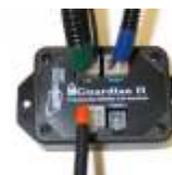
Finally, snap the Vehicle 1 Harness into the Guardian II Module connector labeled in orange “Vehicle 1”.
