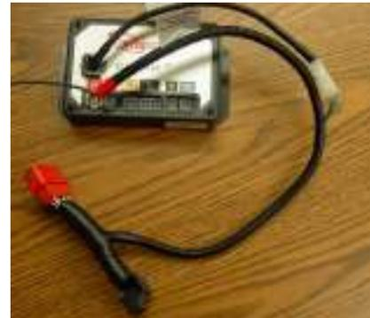
**ILIS Harness** - This harness contains the battery power, vehicle secure, and lift door circuits. The mating harness is to be fabricated by the installer. The recommended mating connector is Molex Part # 0050841040. The recommended mating terminals are Molex Part # 0002081003. The recommended terminal extractor tool is Molex Part # 0011010168. The recommended hand crimp tool is Molex # 0638116800.
