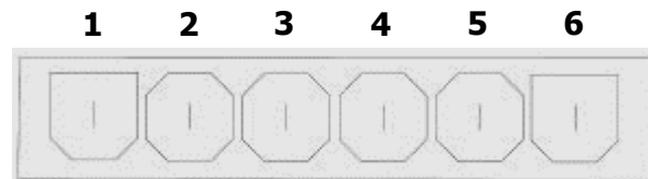
Pin Numbers for the mating connector looking from the back (wire side)
