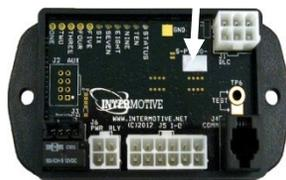
Pin #4 (Gray wire) of the 12 Pin Connector is an auxiliary battery voltage monitor input. It measures the analog battery input and can trigger a low battery restart when this input falls below a user defined level. By default, this trigger is disabled, but it may be enabled via a laptop connection. Contact InterMotive for details or refer to Eco-Star Application Note. A spare Molex pin is provided in the kit to allow the use of this input.
