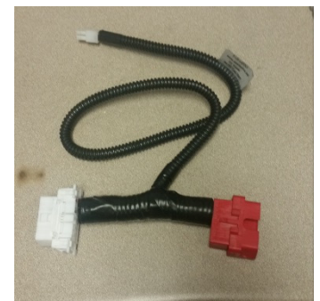
AIM Data Link harness "T's" into OBDII connector.
